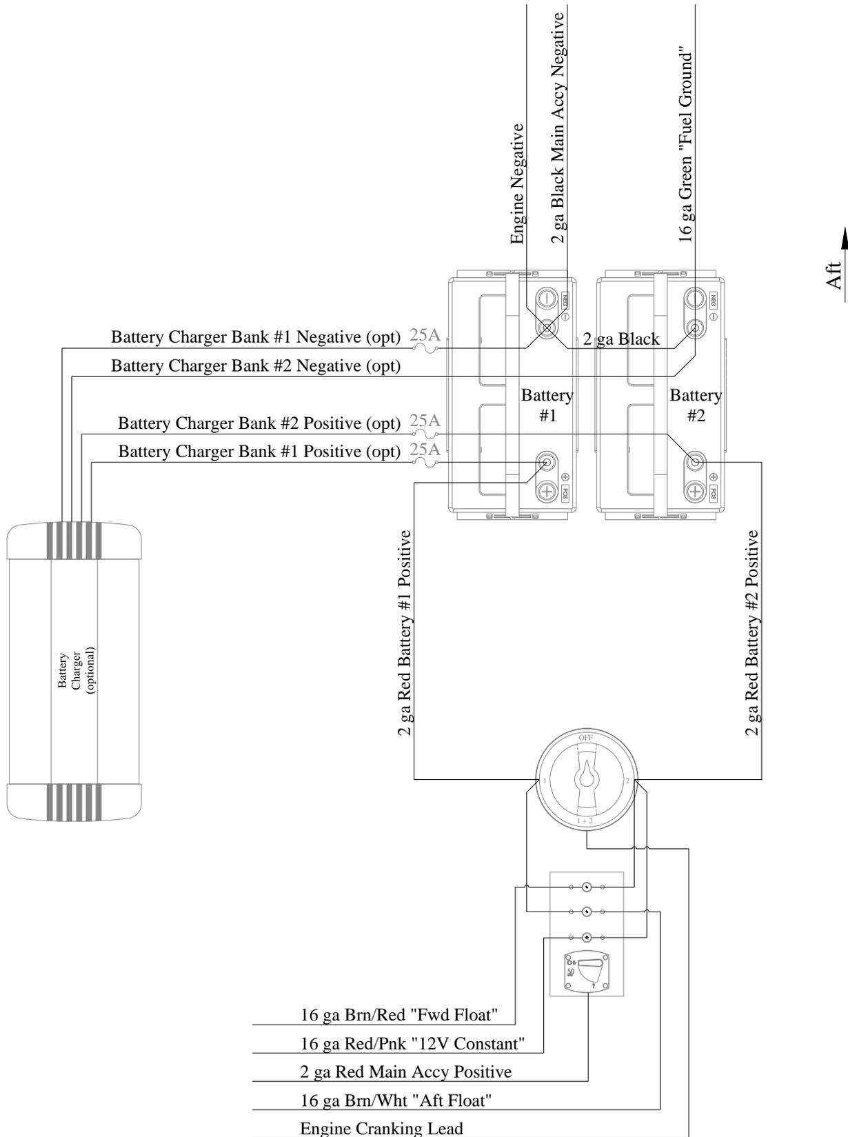
*Battery Wiring with Select Switches - Dual*
